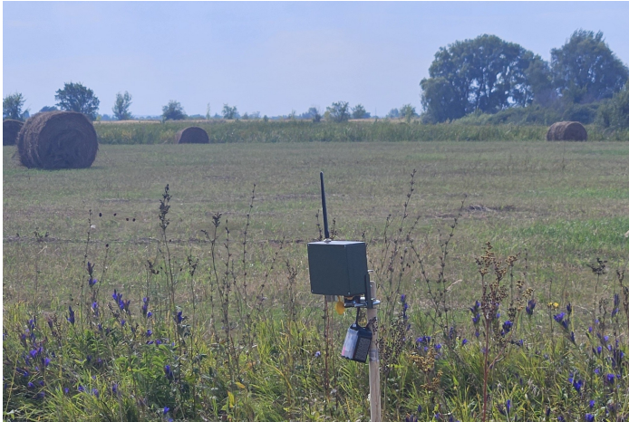
Figure 3. An Alisum-S detector node in a field test posted on 13 Oct. The vendor said five detectors passed alerts through a MESH network to a smartwatch inside a vehicle, with the nearest node about 1 km away and the farthest beyond 2.5 km. These are self-reported test conditions.
