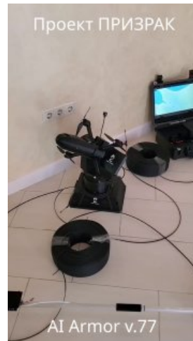
Figure 6. Video thumbnail of the AI Armor v.77 setup posted 15 Oct. The visible equipment includes a control display, launch hardware and a fibre spool; the post also claims acoustic and optical detection.
